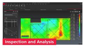
Control Floor Flatness and Levelness (ASTM E1155). Inspect tunnels, roadways and more and produce comprehensive reports for immediate analysis or delivery to stakeholders.
