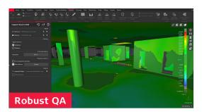
User-defined tolerances for accuracy and precision are analysed and delivered to users for quick, visual QA checks or thorough client reporting.
